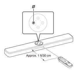
Point the remote control of the TV at the remote control sensor of this unit and press the remote control button to be learned (e.g. the button to increase the volume) 3 times.
